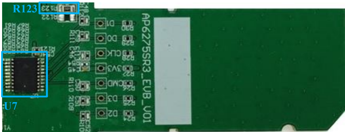
Figure3. EVB interface to HOST SDIO 2.0.
